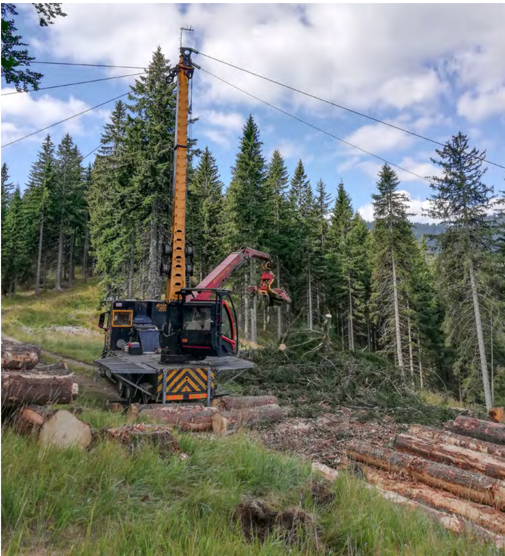
Picture 4: Slope harvester with suspension ropes for optimized harvesting in mountain areas
